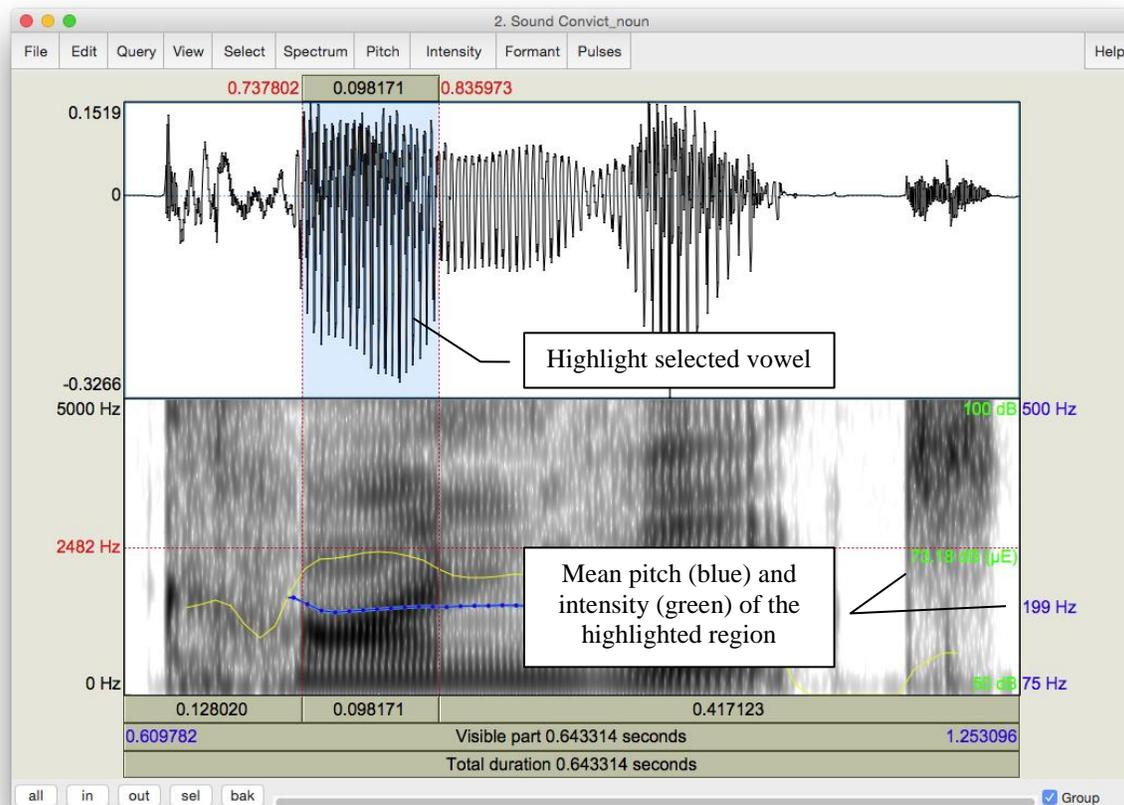
Figure 9.1 Measuring mean pitch and intensity in Praat
