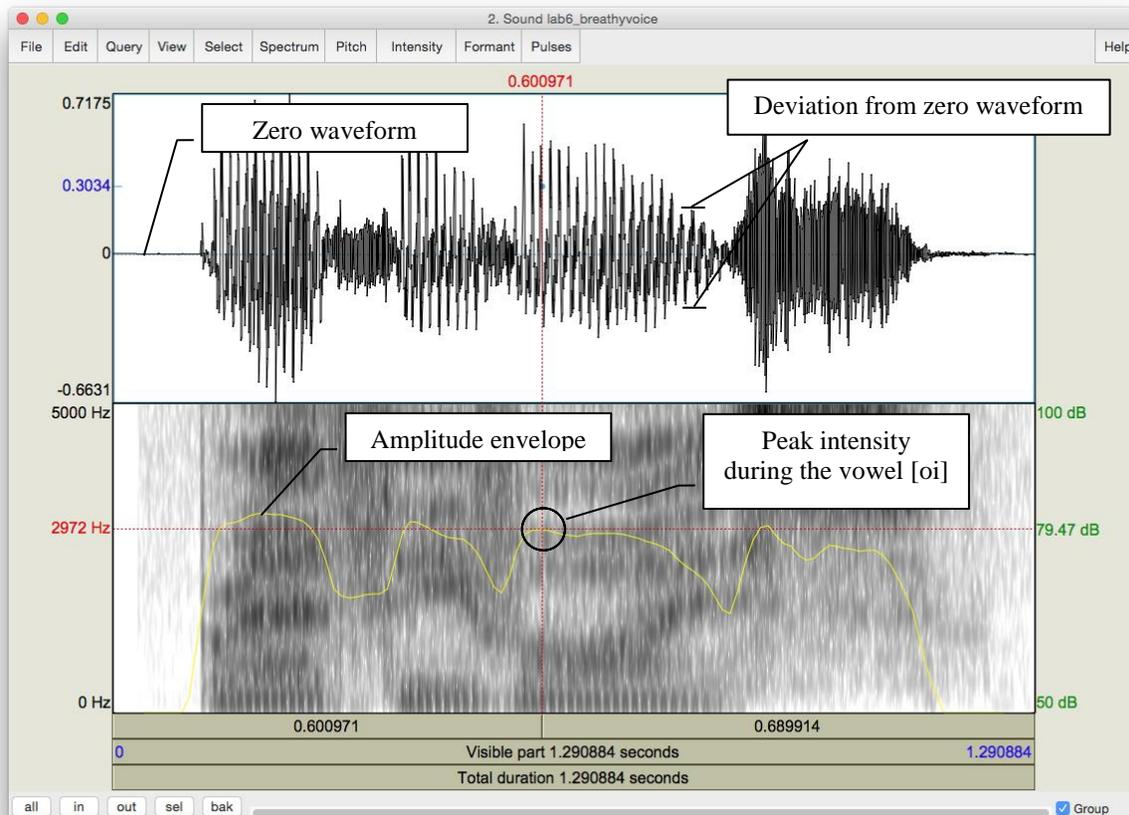
Figure 8.4 Acoustic intensity
