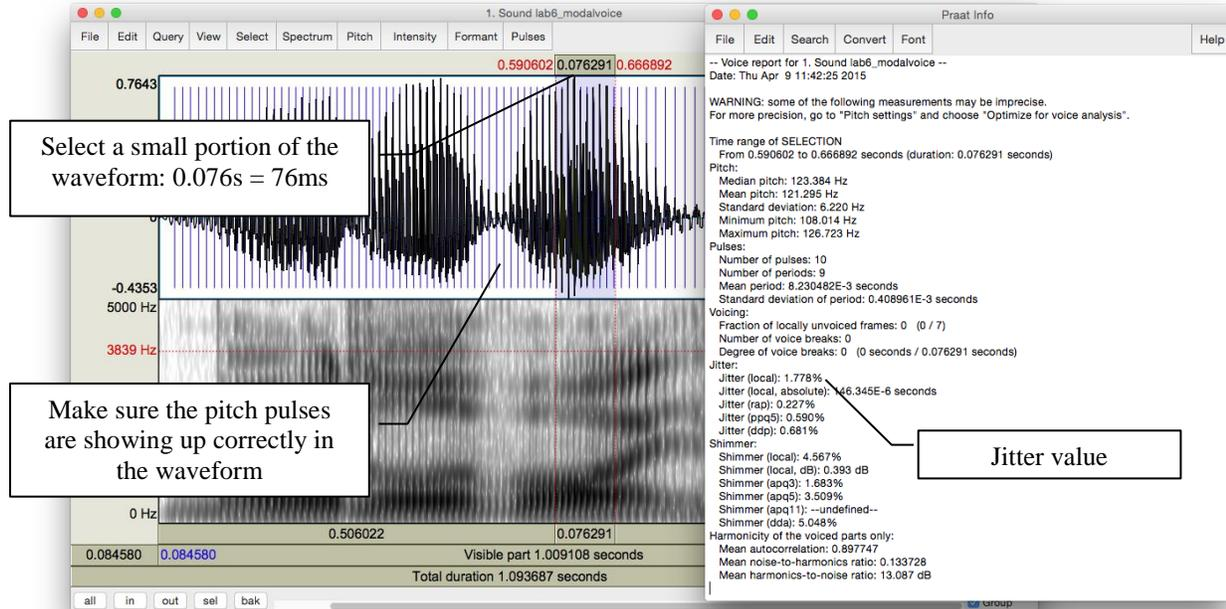
Figure 8.2 Jitter measurement
