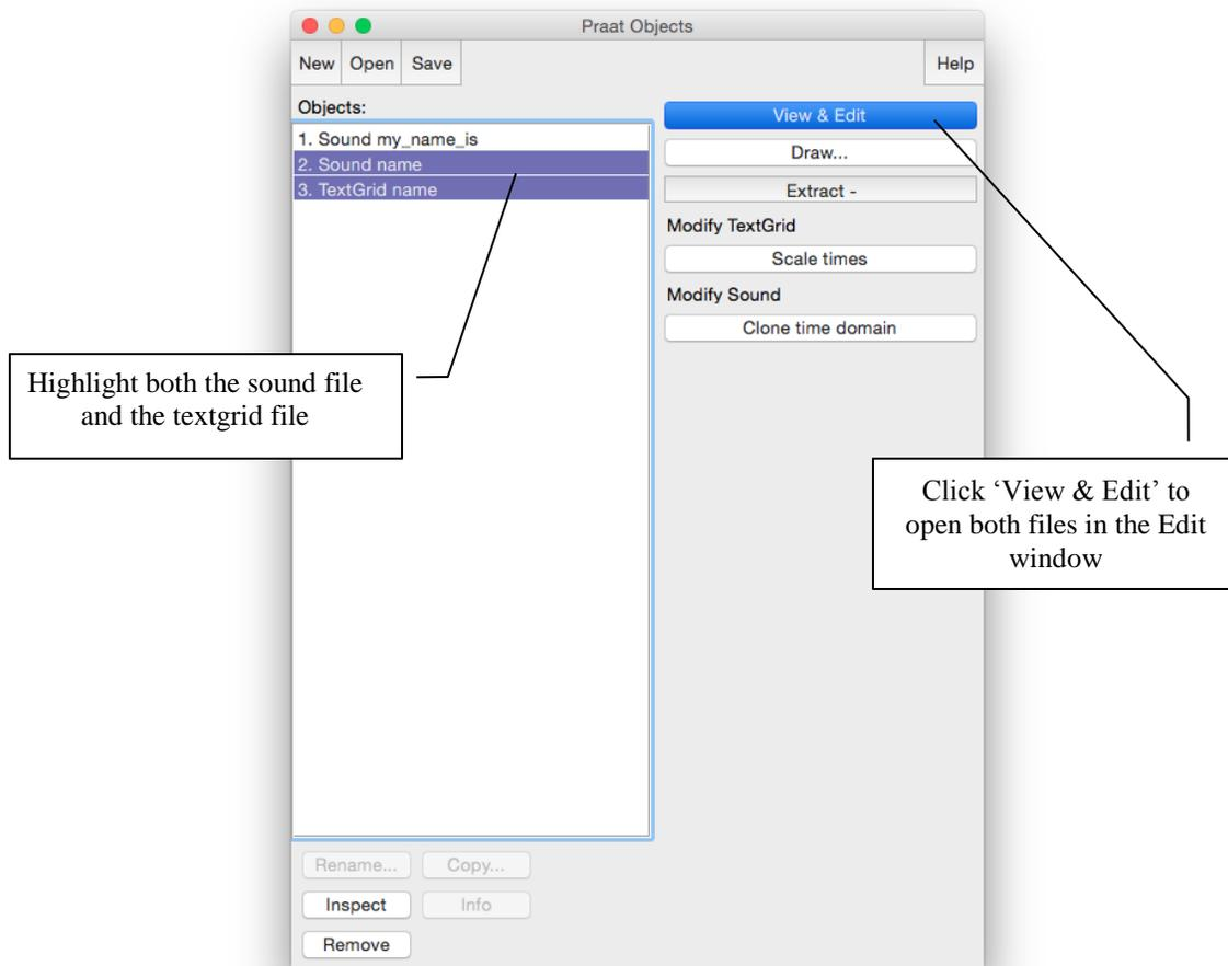
Figure 1.8 Opening a textgrid file with its corresponding sound file
